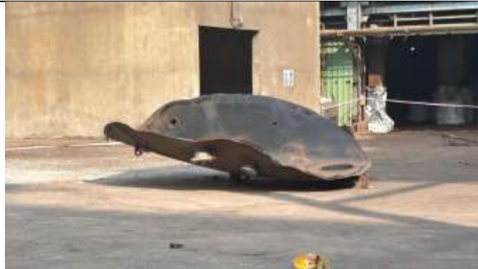
Top of the tank blast off and fell on ground nearby
